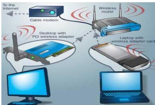
Fig.1: Wireless router connection
