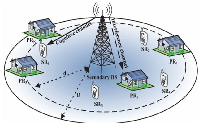
Fig. 1: System model of CR-based cellular network with secondary BS, multiple PRs, and multiple SRs
