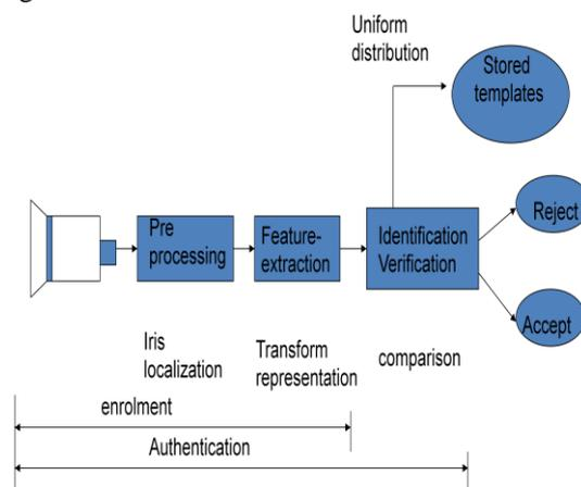
Fig.6 Typical iris system configuration
