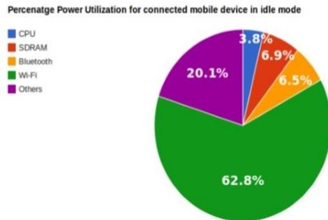
Fig.1: Percentage of power consumption for the connected mobile device in idle mode
