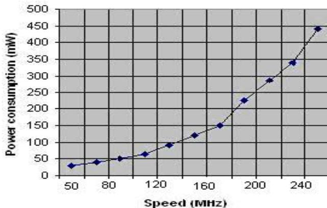
Fig .1: Power consumption in dynamic voltage scaling
