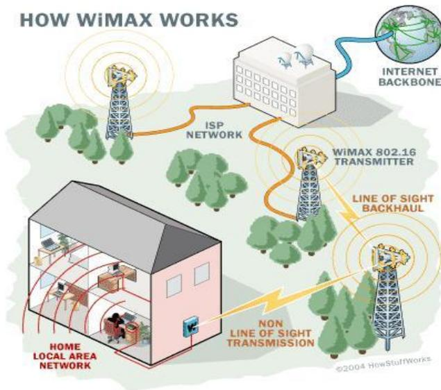
Fig.3: WiMax Working Structure
