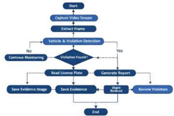
Fig. 6: Activity Diagram of Smart Traffic Violation Detection and Reporting System
