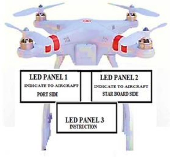
Fig.3.1: Configuration of LED Display (a) from the view with Forward Movement of Aircraft (b) From the Drone view Welcoming Position
