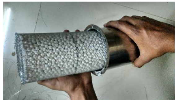
Fig.14: Wire mesh loaded into the chamber
