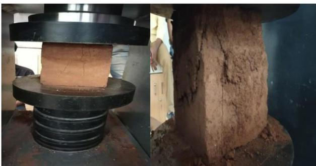
Fig. 8: Testing of Air Cured Samples
