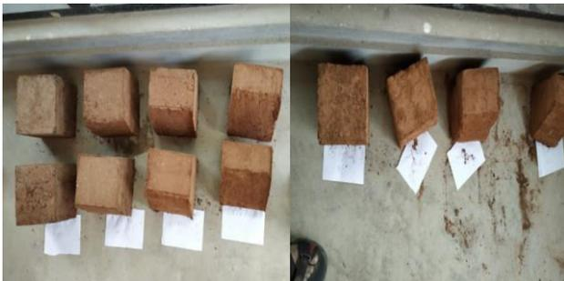
Fig. 7: Blocks Casted and Air Curing
