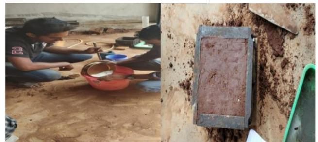
Fig. 6: Red Soil and Sodium Meta Silicate Mixing and its Sample
