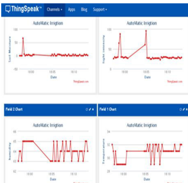
Fig.9: Deployment in Thingspeak cloud for measuring Soil moisture level, humidity, temperature and light intensity
