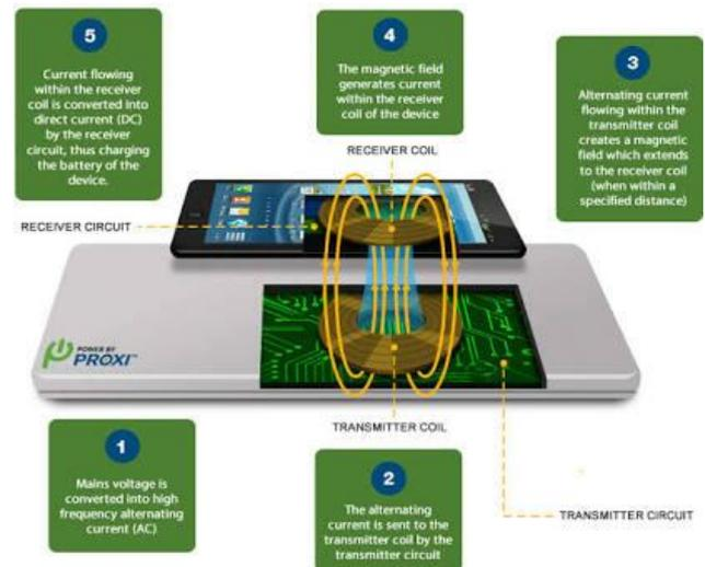
Fig. 3: Wireless Circuit
