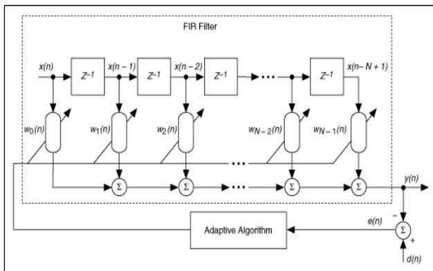
Fig. 7: Adaptive beam forming Algorithm
