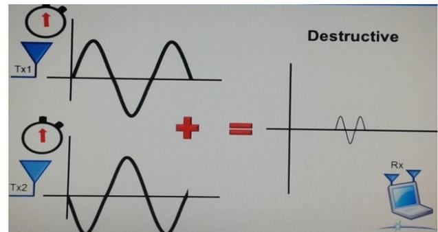
Fig. 1: Destructive in beam forming
