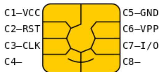
Fig.3: Pin diagram of the Smart Card
