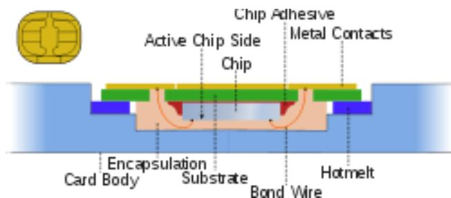
Fig.2: Structural Design of Contact cards
