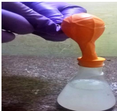
Fig.5: showing the bulged balloon 24 hours after inoculating the fermenting flora. The circumference of the balloon is measured with the help of a thread
