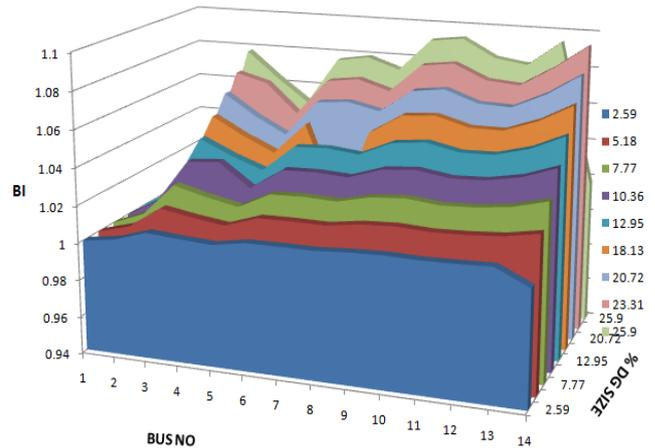
Fig 1: Relation between BI, Bus no, %DG size for 14 bus system.
