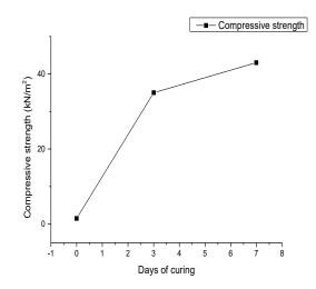
Fig. 9: Number of Days of Curing Versus Compressive Strength For Type 1 Blocks.(Soil 96%+Alccofine 4%)
