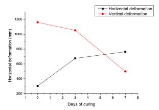
Fig. 10: Number of Days of Curing Versus Deformation For Type 1 Blocks.(Soil 96%+Alccofine 4%)
