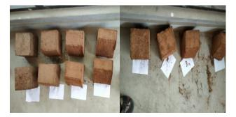
Fig. 7: Blocks Casted and Air Curing
