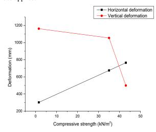
Fig. 11: Compressive Strength Versus DeformationFor Type 1 Blocks.(Soil 96%+Alccofine 4%)
