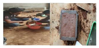
Fig. 6: Red Soil and Sodium Meta Silicate Mixing and its Sample
