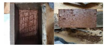
Fig. 4: Scratching and Soil Sample Preparation
