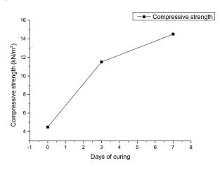
Fig. 12: Number of Days Versus Compressive StrengthFor Type 2 Blocks.(Soil 97%+Sodium Meta Silicate 3%)
