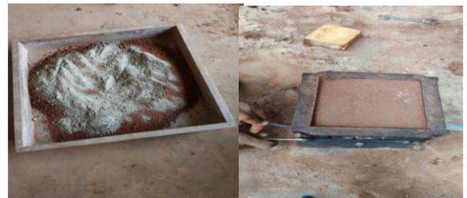
Fig. 5: Soil Plus Alccofine Mixing and its Sample
