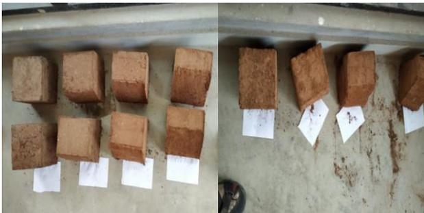
Fig. 7: Blocks Casted and Air Curing
